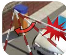
Arm automatically swing out or auto reverse when hitting vehicle to minimize damage. Optional rubber lining or photobeam can be added to further enhance safety level.
